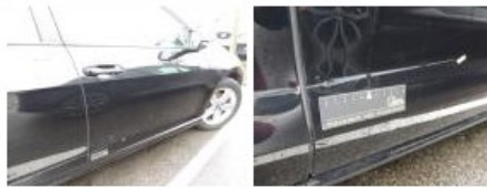
Door R R, Bump(s) and scratch(es), LI - Repair and paint (complete) 510,35
