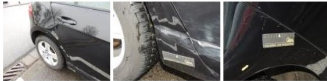
Door F R, Bump(s) and scratch(es), LI - Repair and paint (complete) 414,35
