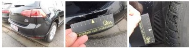
Wing R R, Bump(s) and scratch(es), LI - Repair and paint (complete) 548,20
