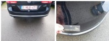
Bumper R, Scratch(es), It - Spot repair 115,56
