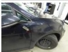
Wheel cover F R, Missing, E - Replace
