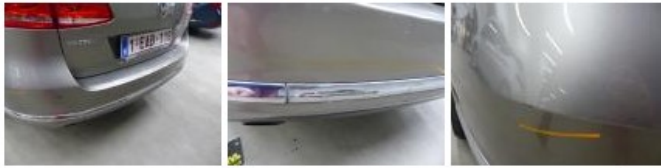
Wing R L, Bump(s), LI - Repair and paint (complete) 380,20
