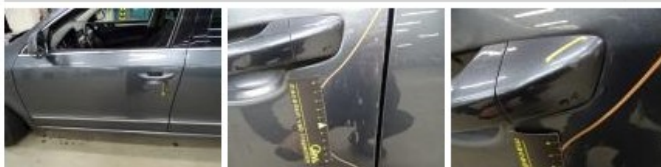
Door F L, Scratch(es), LI - Repair and paint (complete) 382,02
