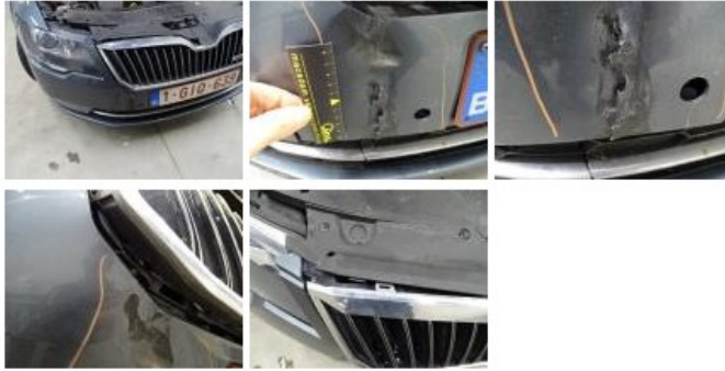
Bumper R, Scratch(es), LI - Repair and paint (complete) 254,16
