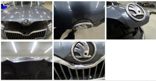
Front bumper, Damaged, Le - Replace and paint 862,80
