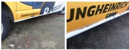
Door F R, Scratch(es), LI - Repair and paint (complete) 286,76
