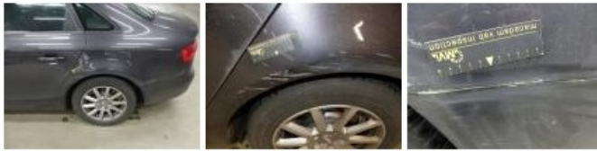
Wing F L, Bump(s) and scratch(es), LI - Repair and paint (complete) 220,18
