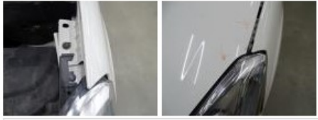
Wing F L, Incomplete, E - Replace 20,00
