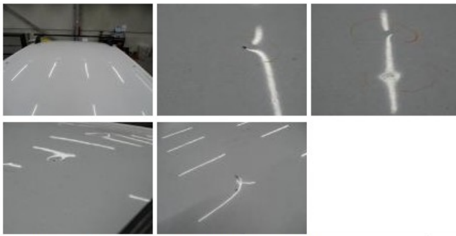
Trunk door R R, Bump(s) and scratch(es), It - Spot repair 115,56
