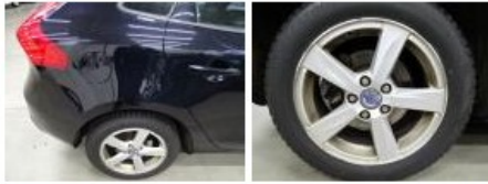
Wing R R, Scratch(es), LI - Repair and paint (complete) 95,00
