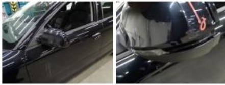
Door R R, Scratch(es), LI - Repair and paint (complete) 318,35
