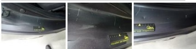
Rocker panel inner R R, Bump(s) and scratch(es), LI - Repair and paint (complete) 115,56
