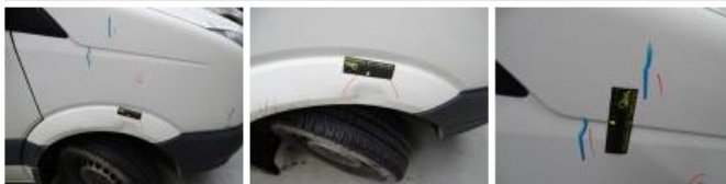
Wing F R, Bump(s) and scratch(es), LI - Repair and paint (complete)
