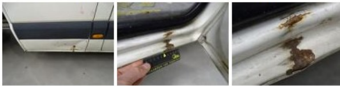
Sill outer R, Bump(s) and scratch(es), LI - Repair and paint (complete)
