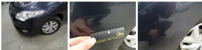
Front bumper, Stone chip(s), LI - Repair and paint (complete)
