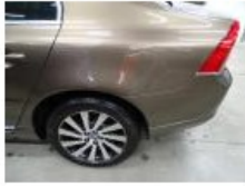
Alloy rim R L, Scratch(es), LI - Repair and paint (complete) 95,00
