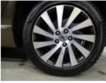
Alloy rim R L, Scratch(es), LI - Repair and paint (complete) 95,00
