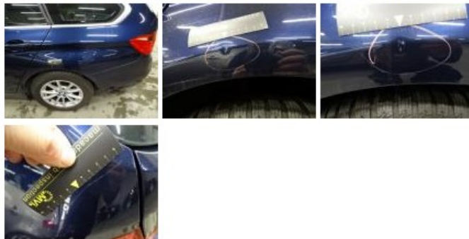
Door F R, Bump(s) and scratch(es), LI - Repair and paint (complete) 318,35
