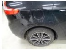
Bumper R, Scratch(es), LI - Repair and paint (complete) 211,80
