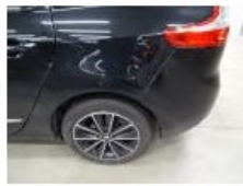
Sill outer L, Bump(s) and scratch(es), LI - Repair and paint (complete) 310,50
