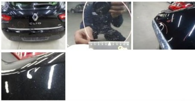
Bonnet, Chemical polution, LI - Repair and paint (complete) 232,06
