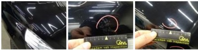
Wing R L, Scratch(es), LI - Repair and paint (complete) 246,56
