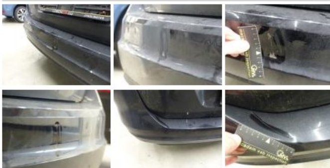
Front bumper, Bump(s) and scratch(es), LI - Repair and paint (complete)
