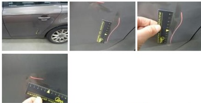
Wing F L, Bump(s) and scratch(es), LI - Repair and paint (complete) 220,18
