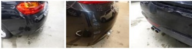
Bumper R, Bump(s) and scratch(es), Le - Replace and paint 766,80
