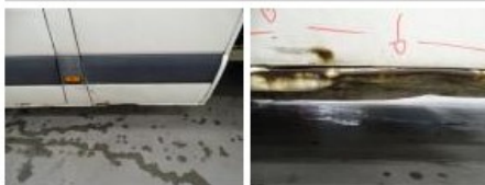
Door R L, Bump(s) and scratch(es), LI - Repair and paint (complete)
