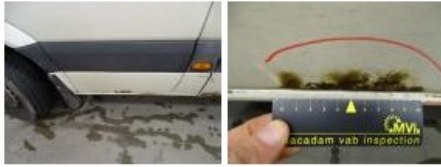
Wing R L, Hole, LI - Repair and paint (complete)
