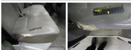
Sill outer L, Bump(s) and scratch(es), LI - Repair and paint (complete)
