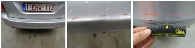
Bumper grille, Damaged, E - Replace
