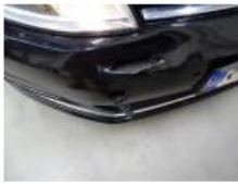
Bonnet, Bump(s) and scratch(es), LI - Repair and paint (complete)
