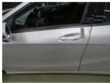
Door F L, Bump(s) and scratch(es), LI - Repair and paint (complete) 318,35
