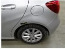
Wing R L, Bump(s) and scratch(es), LI - Repair and paint (complete) 308,20
