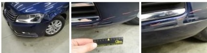
Wing R R, Scratch(es), Acceptable
