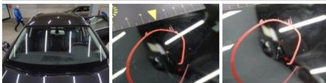
Wing F R, Chemical pollution, LI - Repair and paint (complete)
