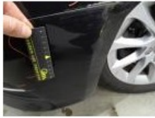
Door F L, Bump(s) and scratch(es), LI - Repair and paint (complete) 318,35
