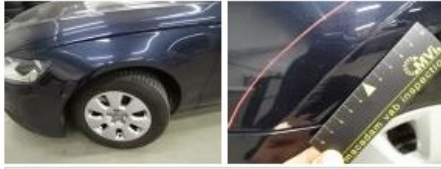
Wing R R, Scratch(es), LI - Repair and paint (complete) 369,84
