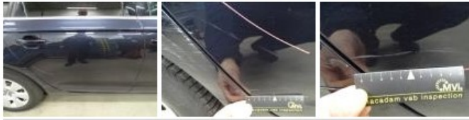
Wing F L, Scratch(es), LI - Repair and paint (complete) 264,21
