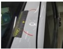
Roof pillar L, Bump(s), LI - Repair and paint (complete)
