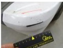
Trunk door R L, Bump(s) and scratch(es), It - Spot repair
