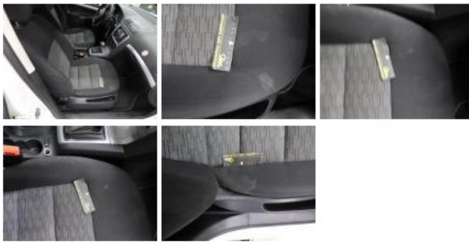
Seat cover R L, Stain, Cleaning
