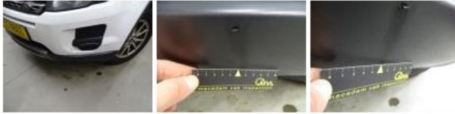
Door F L, Bump(s) and scratch(es), LI - Repair and paint (complete) 382,02
