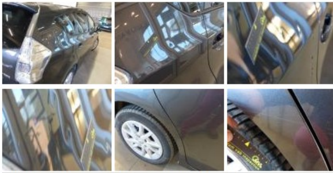
Tailgate, Hail damage, PDR - Knock out without painting
