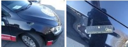
Door R L, Scratch(es), LI - Repair and paint (complete)
