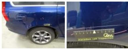
Door R L, Bump(s) and scratch(es), LI - Repair and paint (complete) 382,02
