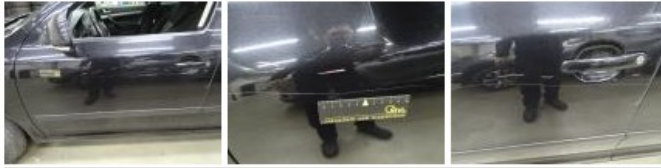
Door R R, Bump(s) and scratch(es), Le - Replace and paint 0,00
