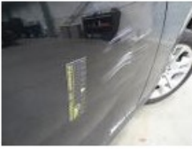
Door F R, Bump(s) and scratch(es), LI - Repair and paint (complete)
