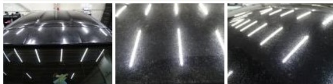
Wing R R, Chemical polution, LI - Repair and paint (complete) 308,20
