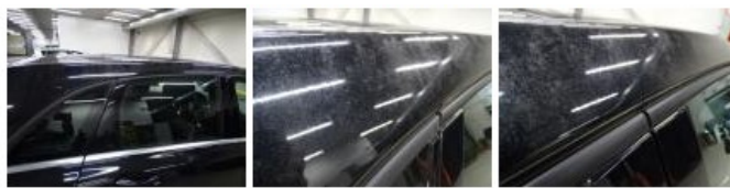
Door F R, Chemical polution, LI - Repair and paint (complete) 318,35
