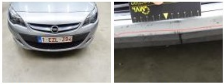
Wing R R, Bump(s) and scratch(es), LI - Repair and paint (complete) 0,00
