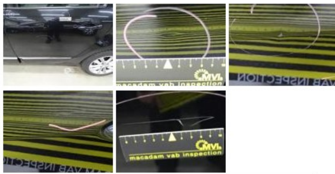
Rocker panel inner F L, Bump(s) and scratch(es), LI - Repair and paint (complete)
