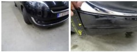
Sill outer L, Bump(s) and scratch(es), It - Spot repair 115,56
