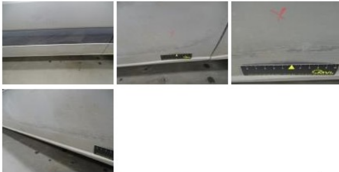
Door moulding Lower R L, Damaged, E - Replace 91,50
