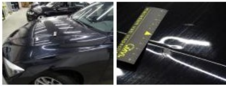
Roof, Bump(s), LI - Repair and paint (complete) 481,50
