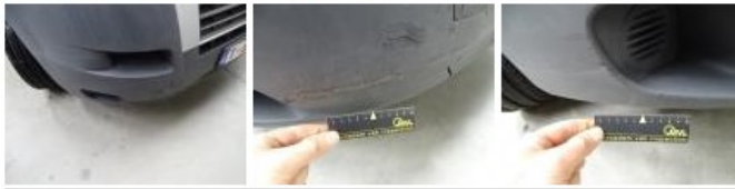
Wheel aperture R R, Rust, Le - Replace and paint 296,00
