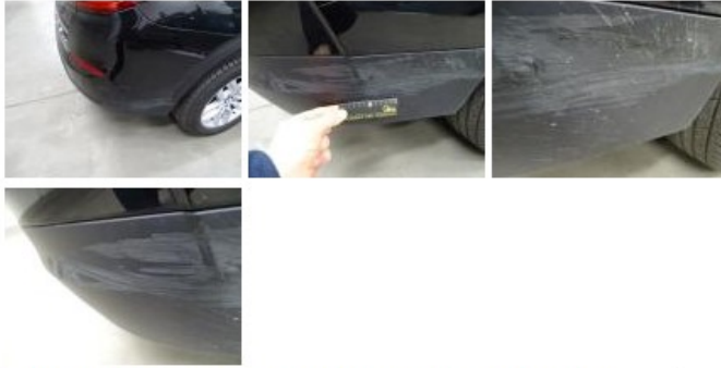
Wing R R, Bump(s) and scratch(es), LI - Repair and paint (complete)
