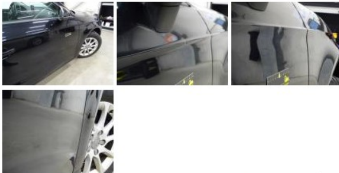
Door R R, Chemical polution, LI - Repair and paint (complete) 318,35
