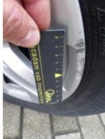
Alloy rim F L, Scratch(es), LI - Repair and paint (complete) 95,00
