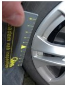
Alloy rim R R, Scratch(es), LI - Repair and paint (complete) 95,00
