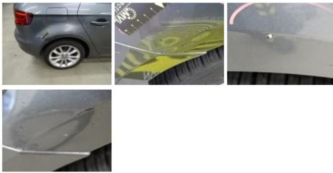
Roof pillar L, Bump(s), LI - Repair and paint (complete) 220,18
