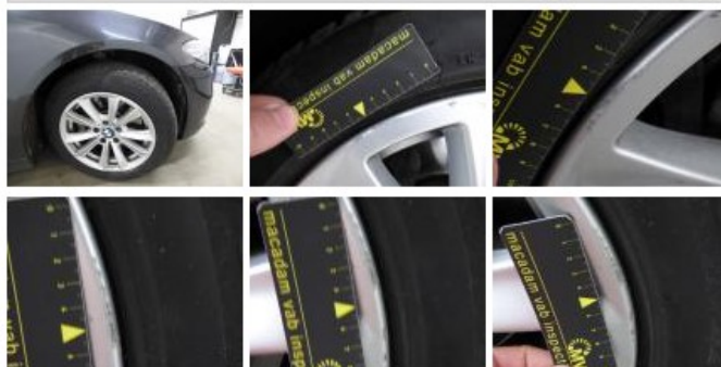
Wing R R, Bad repair, Acceptable
