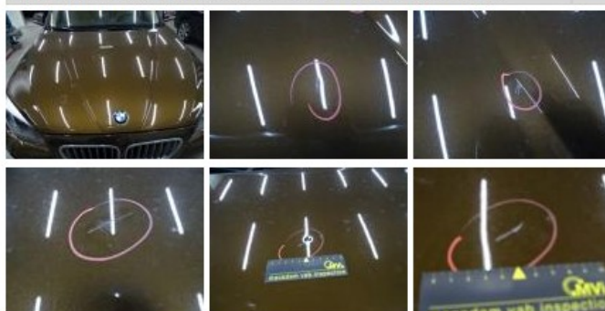
Bonnet, Bump(s) and scratch(es), LI - Repair and paint (complete)
