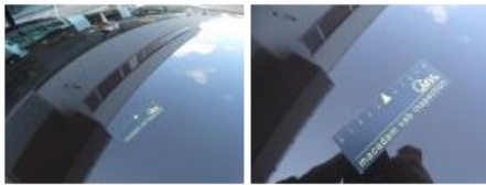
Wing R R, Bump(s) and scratch(es), LI - Repair and paint (complete)
